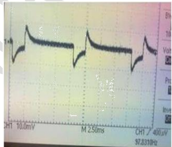
C_{OUT}=2.2\mu F V_{IN}=5V V_{OUT}=3.3V I_{OUT}=10mA to 1A
